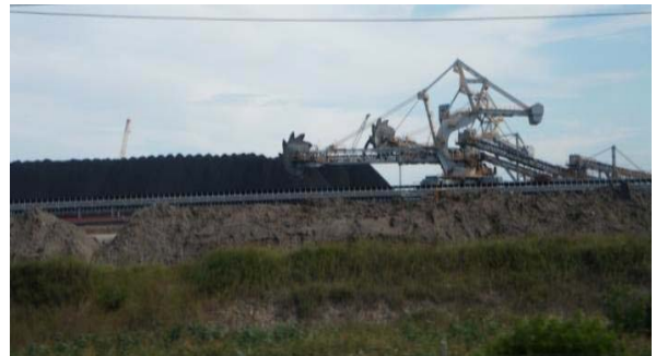
Coal Stockyard: Stacking and reclaiming facilities
