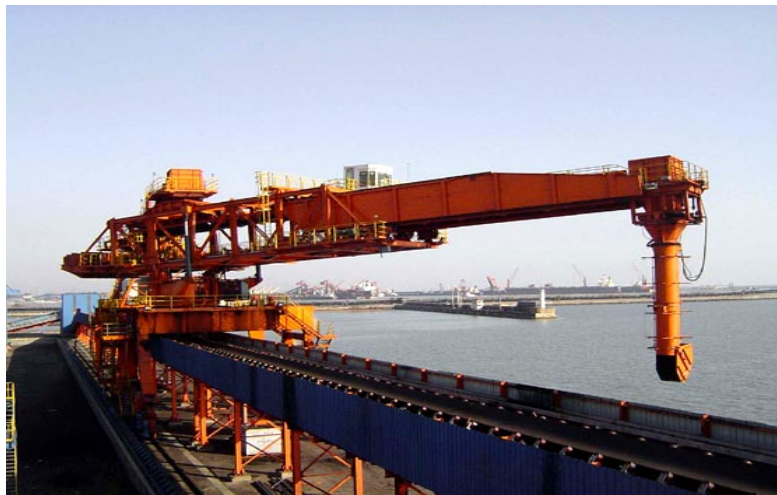
Figure 12.4: Typical Details of Continuous Ship Unloader
