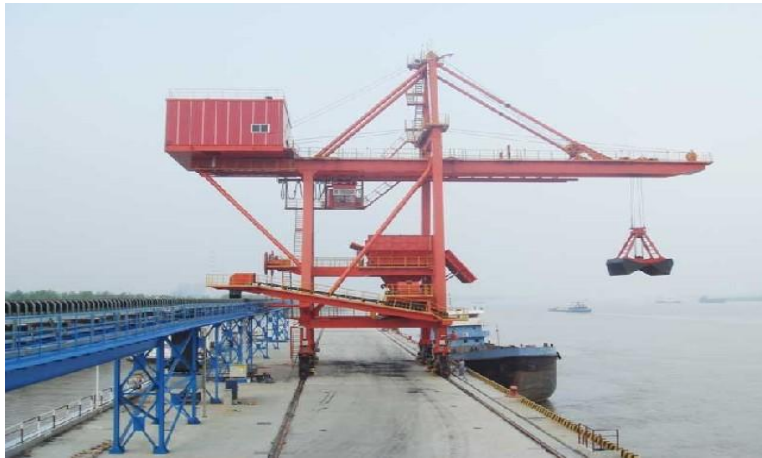
Figure 12.3: Typical Details of Grab Type Ship Unloader
