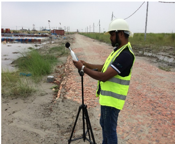
Figure 3.3: Ambient Noise Level Monitoring during Day Time
