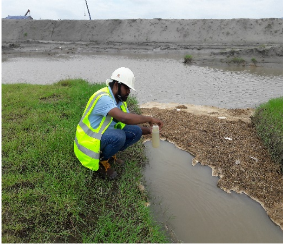
Figure 3.2 (a): Storm Discharge Water Sample Collection
