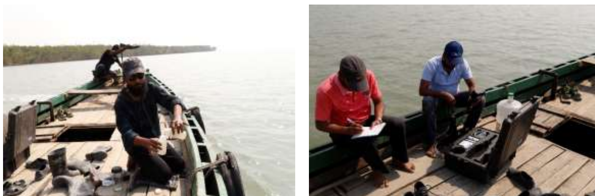
Figure 2.9: Water Sample Collection and insitu Testing of Water Parameters
