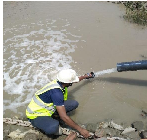
Figure 2.5: RO Discharge outlet and Discharge Water Sample Collection
