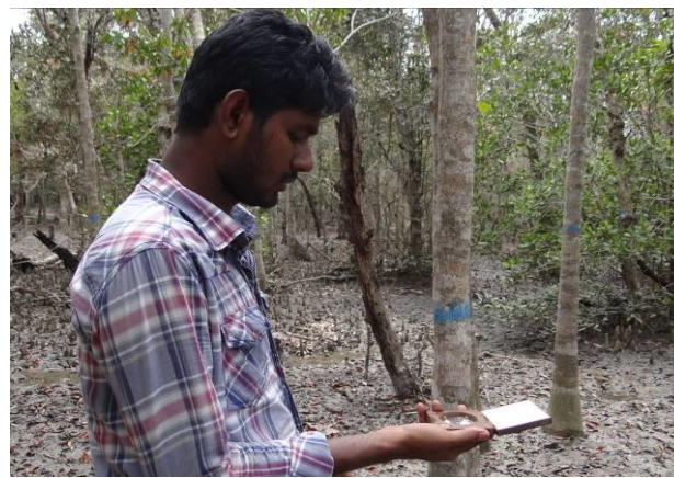
Figure 3.27: Team member taking canopy cover using Lux Meter and Densiometer
