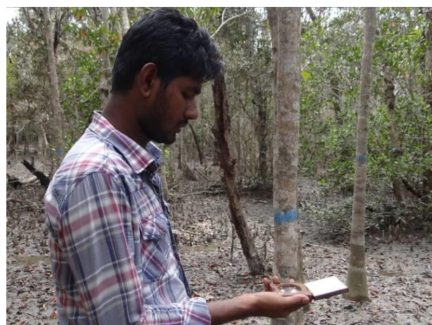
Figure 3.28: Team member taking canopy cover using Lux Meter and Densiometer
