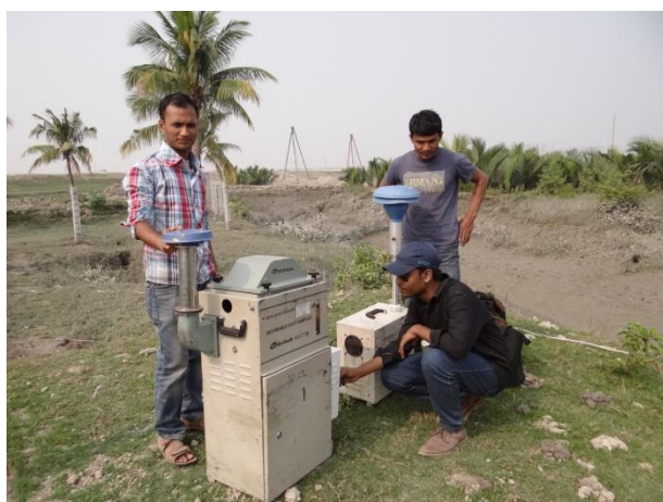
Photo 2.1.1: CEGIS professional checking Air Quality instruments in the Project Township area
