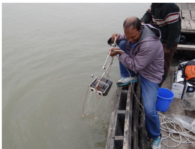
Photo 2.5.1: River bed sediment sampling by Grabber at Project Site
