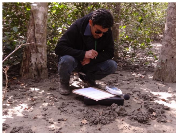
Photo 2.2.2: Professional conducting an ambient noise acquisition survey
