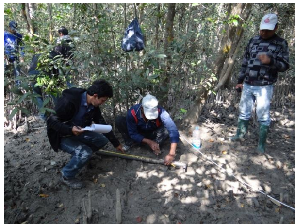
Collecting SRF soil sample by Augering from Akram Point
