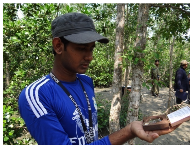
Estimating Tree Height by Laser Range Finder at Akram Point
