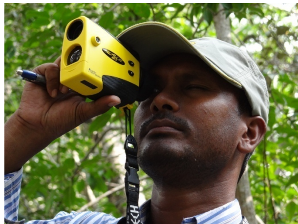
Estimating Tree Height by Laser Range Finder at Akram Point
