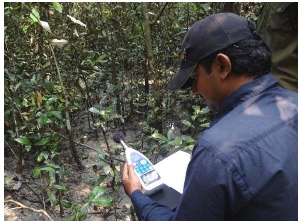
Photo 4.2: Professional conducting an ambient noise acquisition survey
