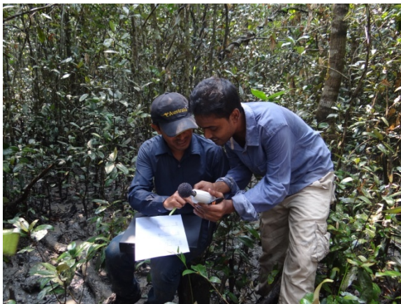
Photo 4.1: Specialists calibrating and setting up noise meter at site before use
