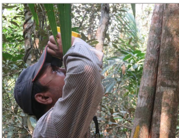
Measuring tree Height at Harbaria by TruPulse 360B Laser Rangefinder
