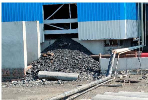
Coal spillage from TP
