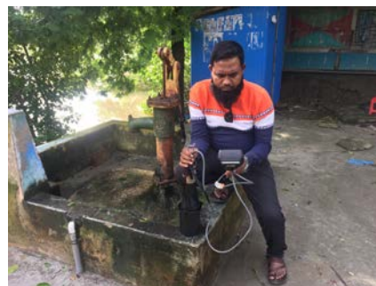
Figure 2.10: Collection and Insitu testing of Groundwater
