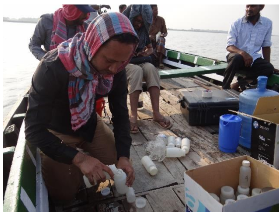
Figure 2.8: River Water Sample Collection, tagging and in-situ testing
