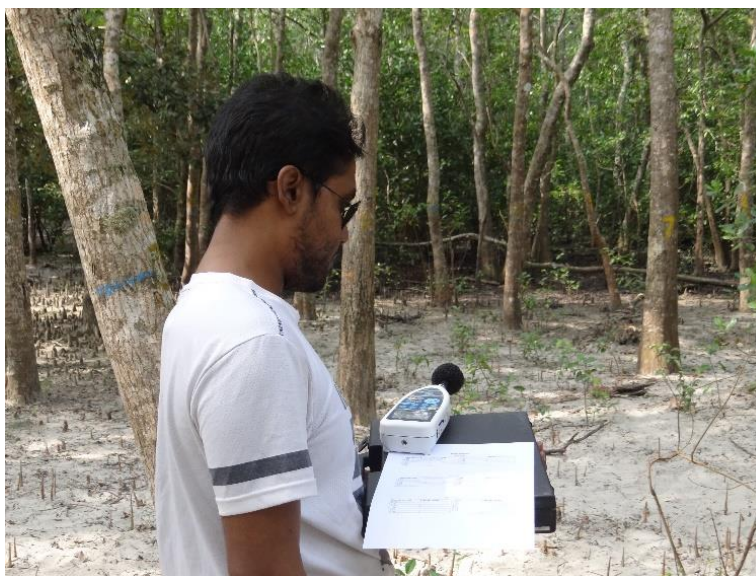
Figure 2.4: Ambient Noise Acquisition in Sundarbans
