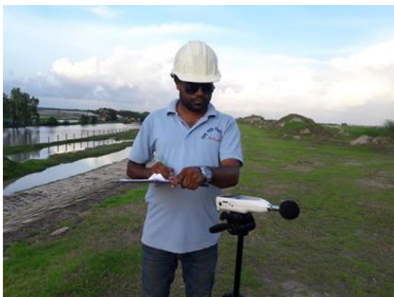
Figure 3.3: Ambient Noise Level Monitoring during Day Time
