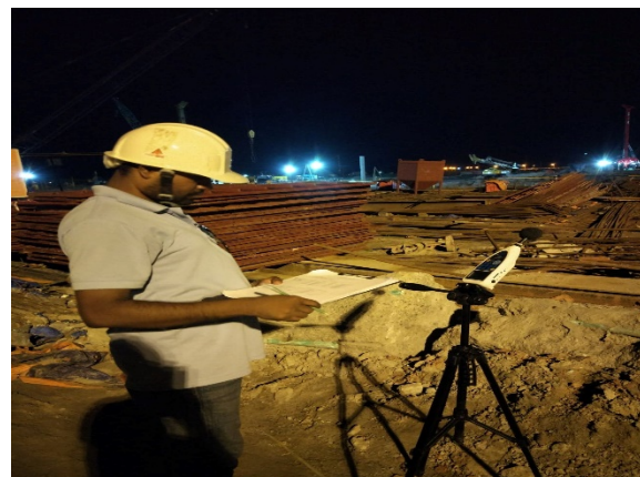
Figure 3.4: Ambient Noise Level Monitoring during Night
