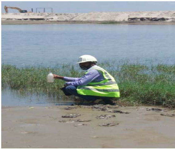
Figure 3.2a: Storm Discharge Water Sample Collection
