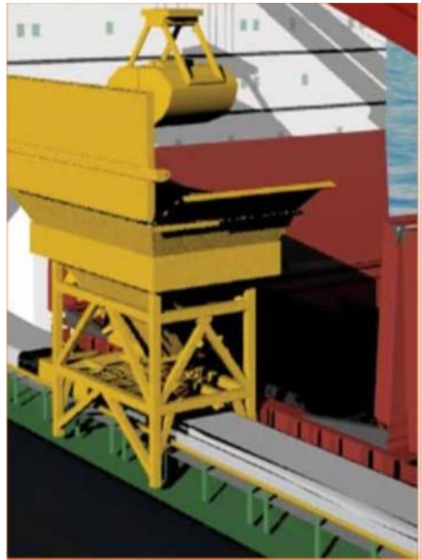
Hoppers designed with anti-spillage plates prevent coal falling into the sea.
