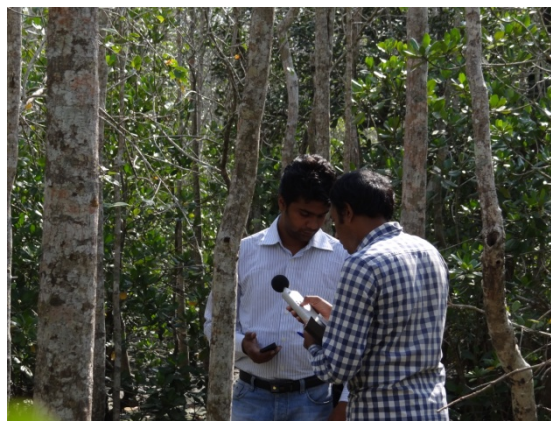
Photo 4.1: Specialists calibrating and setting up noise meter at site before use
