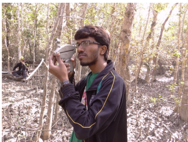
Measuring tree height with The Haga altimeter
